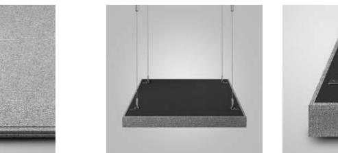
Each panel of the Phonolook Design and Solution line can be installed in **ceiling suspension** by means of **plasticized steel cables** and **threaded clamps**, supplied in the relative fixing kit.
